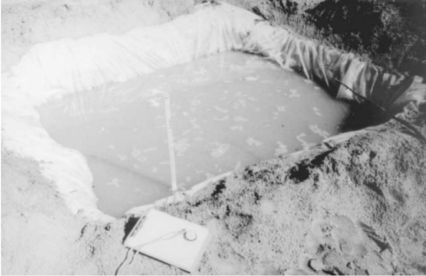
Figure 7.8 Small-scale pilot test basin.
